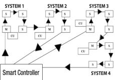
M = Master Evaporator S = Slave Evaporator CU = Condensing unit
